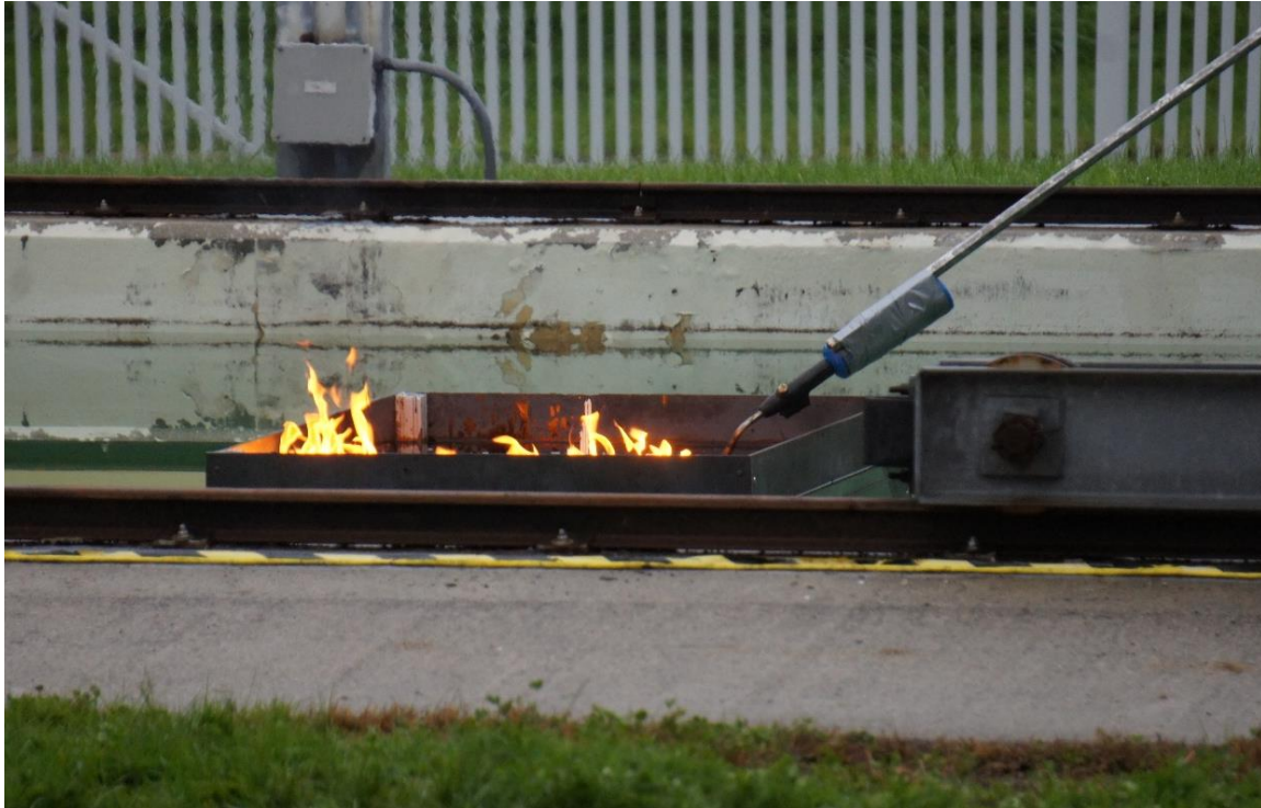
Figure 9. Propane torch ignition of ANS, ~4 cm thickness for all the test burns.
