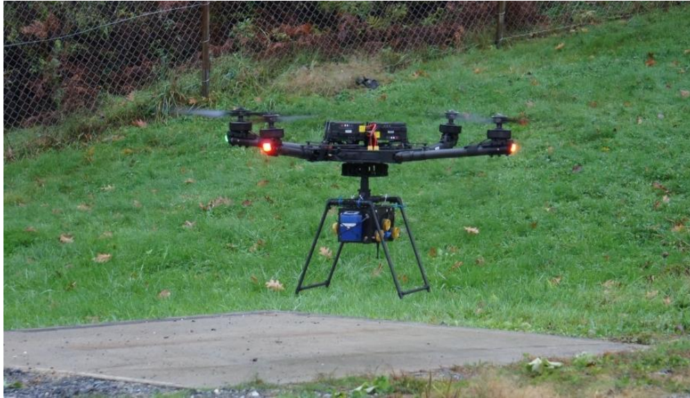
Figure 6. sUAS Freefly Alta X and Kolibri sampling equipment.
