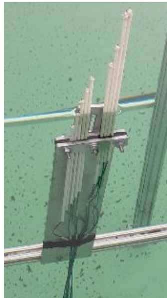
Figure 3. Thermocouple tree in the burn pan before ISB testing.
