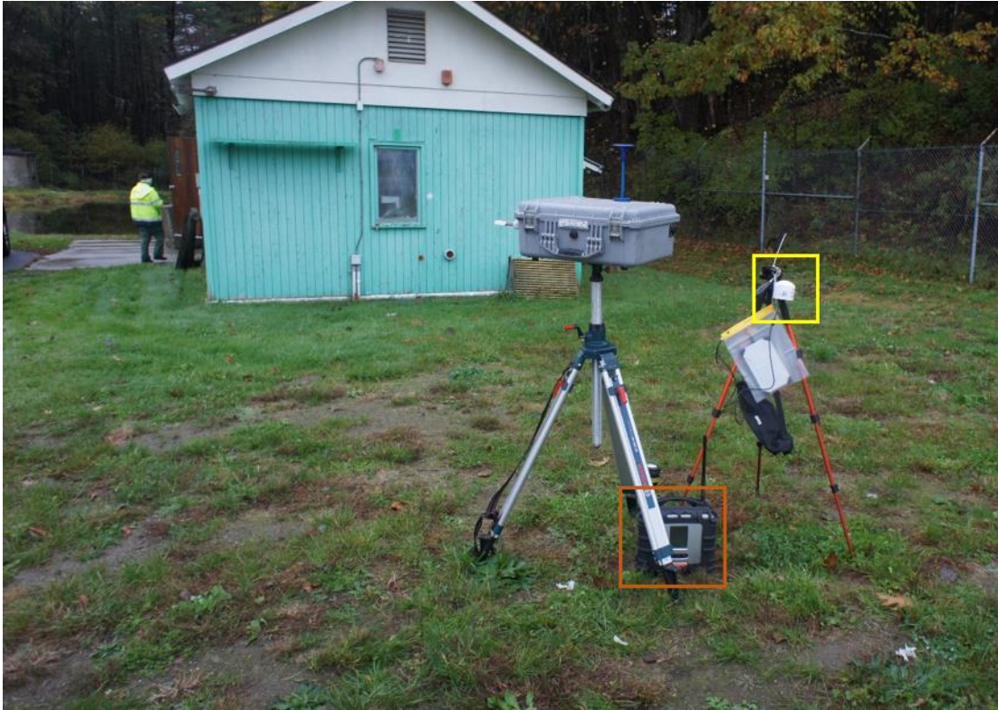
Figure 7. SMART protocol’s DustTrak DRX 8533EP (mounted on tripod) and EPA’s SidePak,(orange square) and PurpleAir (yellow square).
