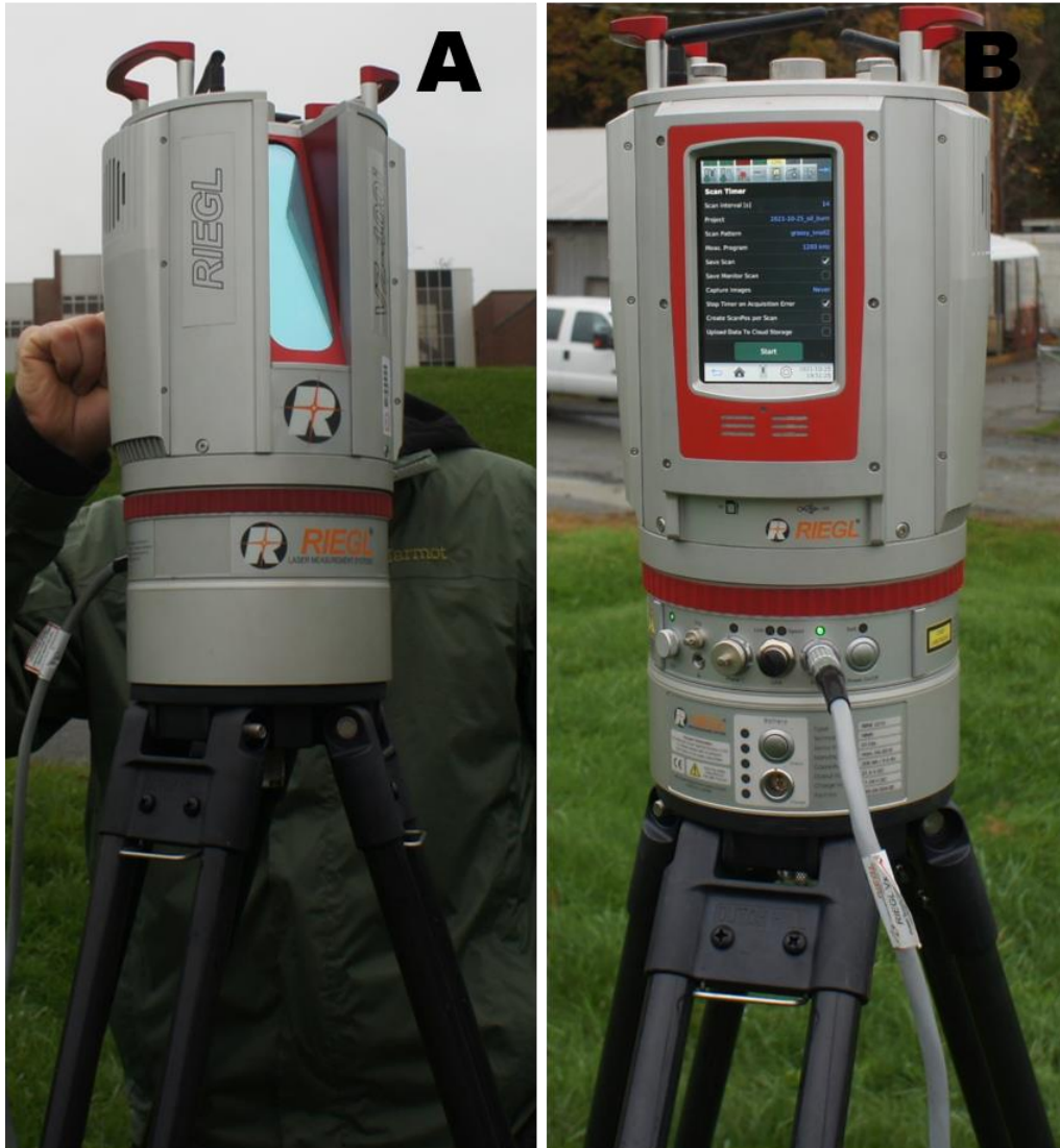
Figure 8. Tripod mounted Riegl VZ 400i and VZ-2000i Terrestrial Laser Scanner.
