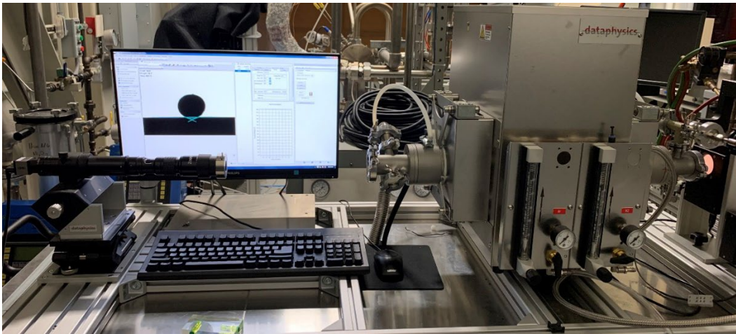
Fig. 2 Contact-angle test measurement setup for a standard sample
