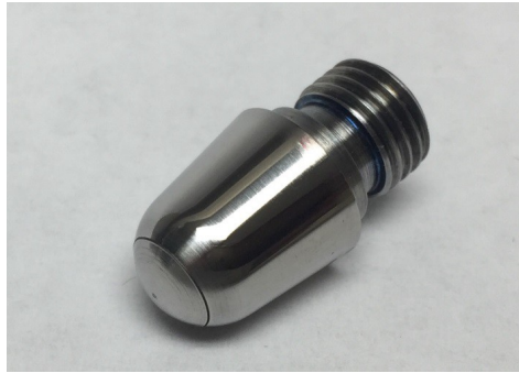
Figure 7-20: Nosetip of R_N = 5.08 mm with 210 Equally Spaced 15 \mu\text{m} Cubical Roughness Elements that Were Laser-Machined Circumferentially at 45^\circ from the Apex of the Spherical Tip.
