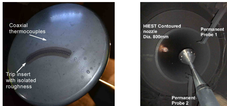
Figure 9-17: Apollo Model with 'Pizza Box' Shaped Isolated Roughness Elements ( k = 0.3 mm) and Model Installation in Hiest Test Section.
