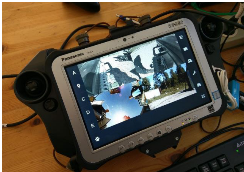
Figure 4-2: A Tablet Computer is Inserted into the Docking Station.
