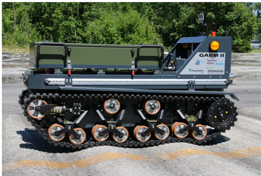
Figure 2-2: Robot Platform, 'Garm' with a Standardized Payload (In This Case a Simple Transport Box).
