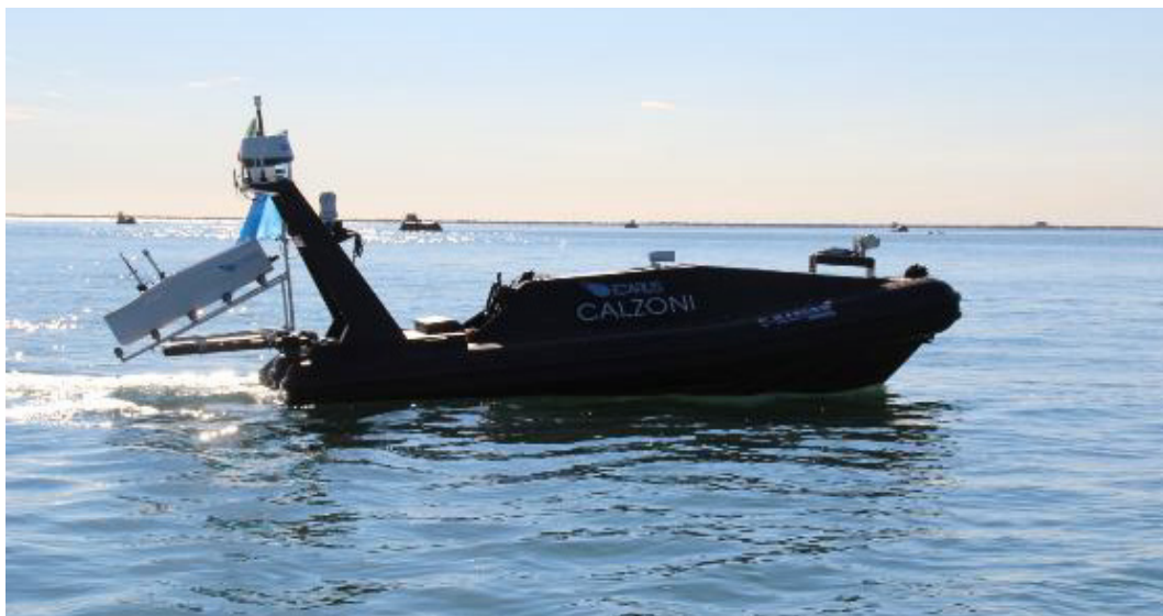
Figure 1-13: Unmanned Surface Vehicle Deploying the Unmanned Rescue Capsule.
