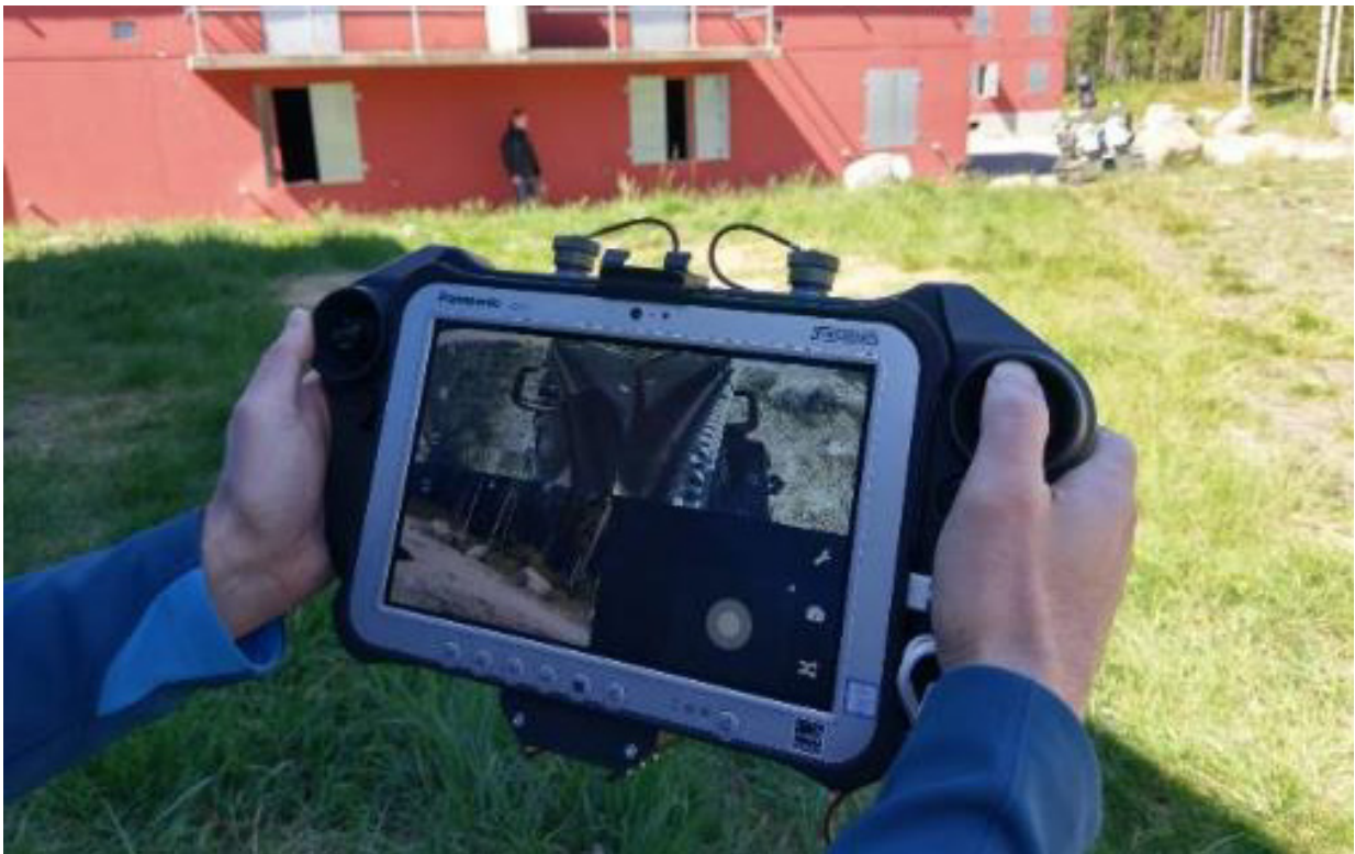
Figure 4-4: Garm Robot, Teleoperation with OCU.
