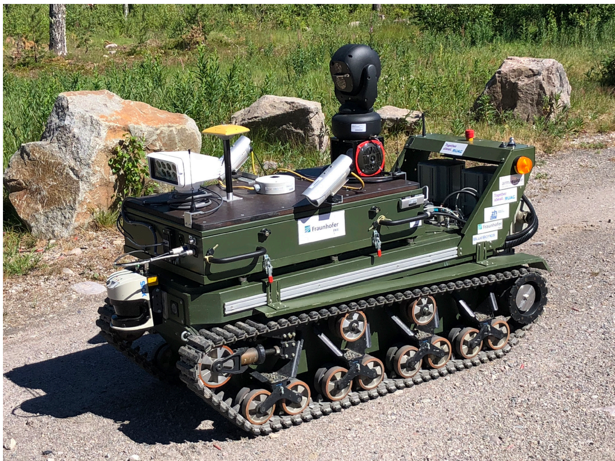
Figure 3-1: Robot Platform, ‘Garm’, with a Reconnaissance Payload.
