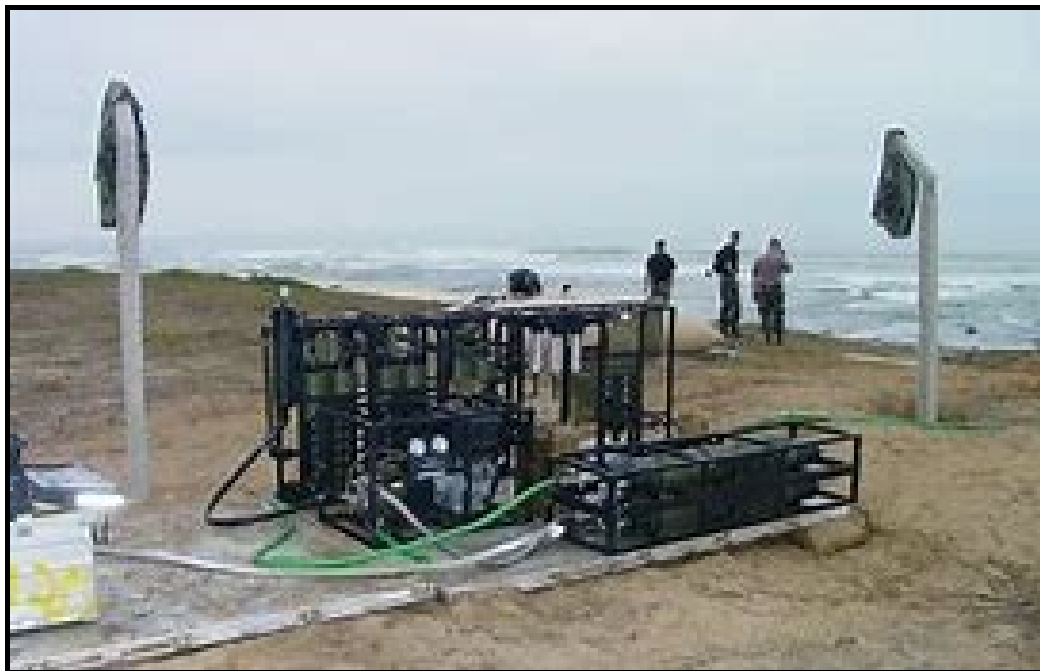
Figure 24: Tactical Water Distribution Equipment System (TWDS).
