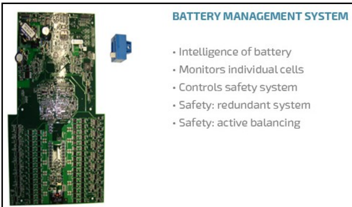
Figure 40: Battery Management System.
