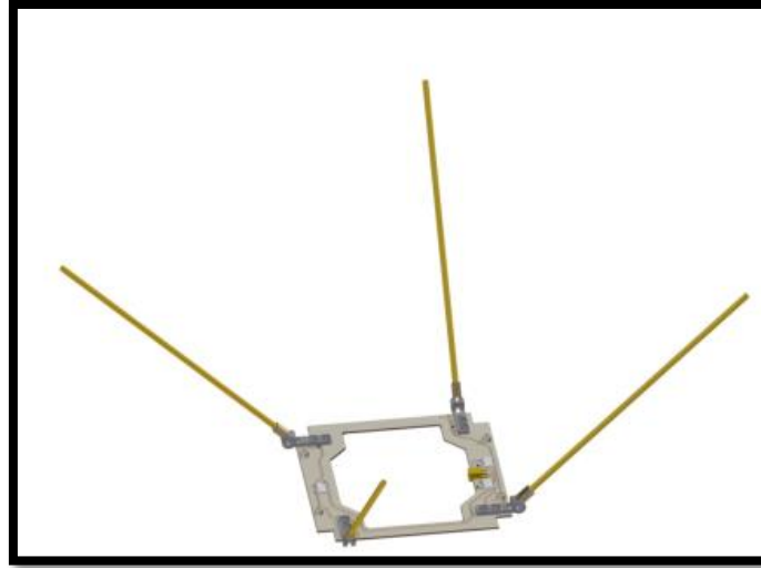
Figure 53. GOMSPACE NanoCom ANT430 Transceiver Antenna
