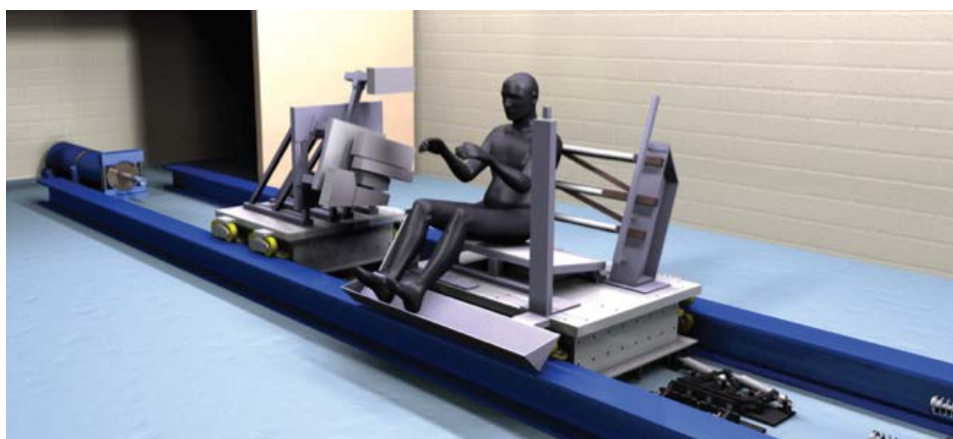
Figure 5-15. Rendering of UMTRI's dual-sled impact facility.
