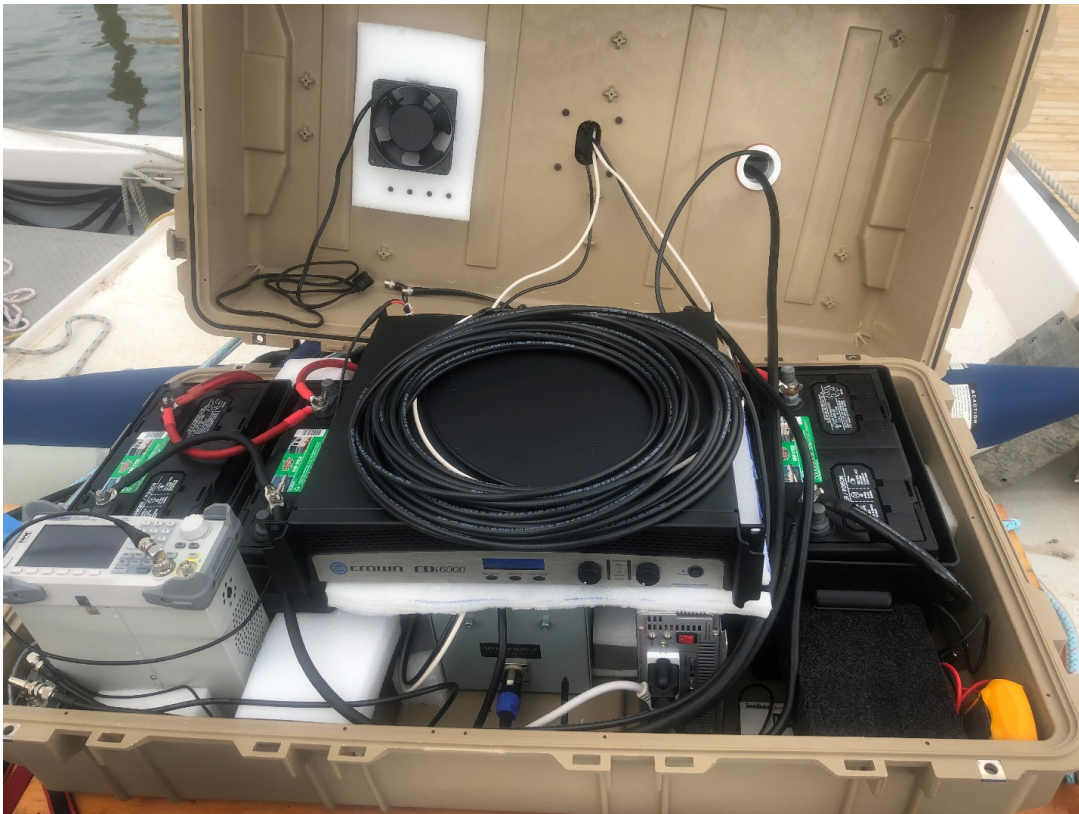
Figure 9 COFFIN interior with waveform generator, three batteries, GPS receiver, amp, inverter, Lubell bridge, and cooling fan.
