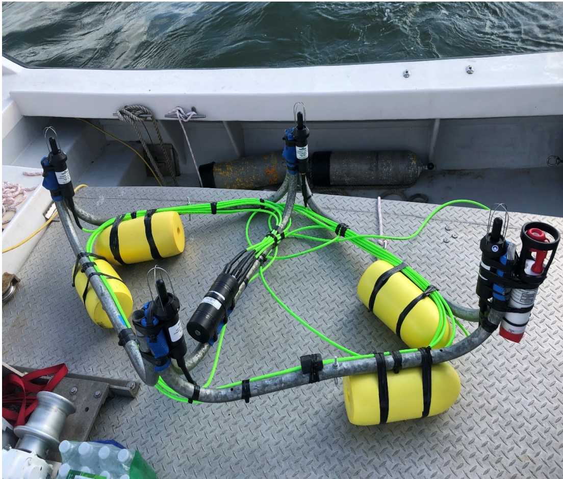
Figure 11 Inverted dBRd prior to deployment with icTalk, icListens, icSync, and RBR visible. Yellow buoys were used to change the depth/maintain the depth of the dBRd system.
