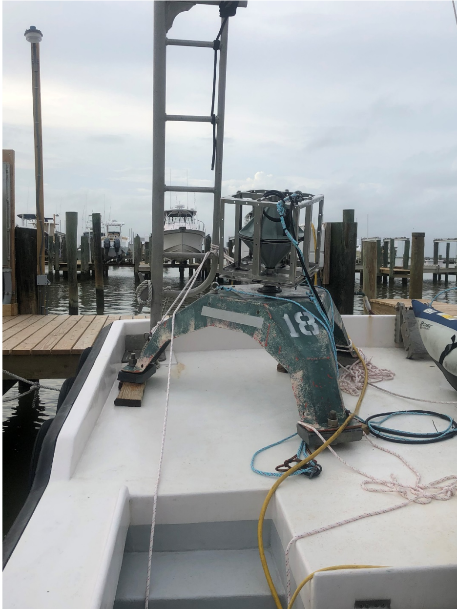
Figure 7 Lubell source on spider. The spider was held in place with 50lb weights bolted onto each leg. A bungy chord was used to ensure the lines would not ensnare the Lubell sound source ability to swivel.
