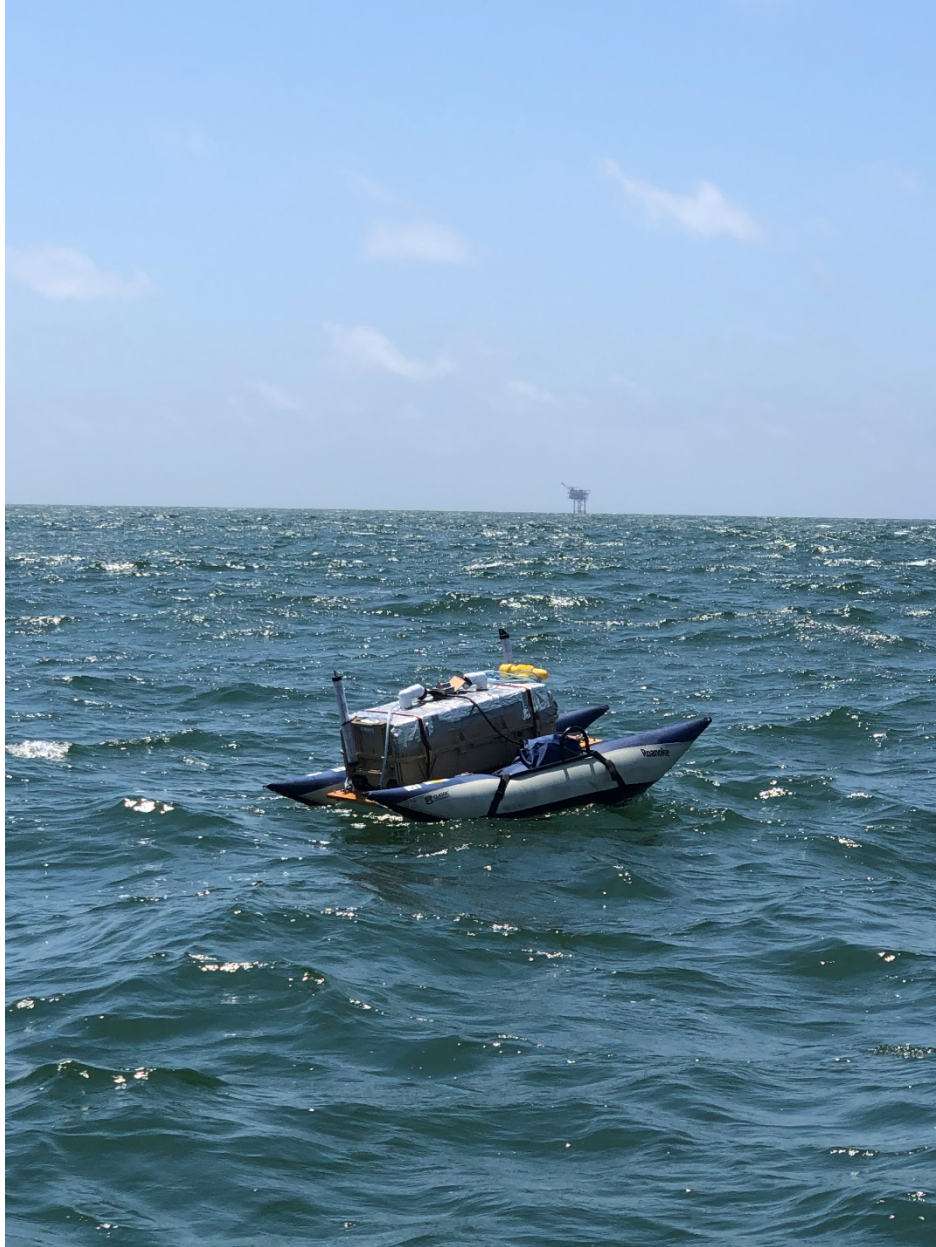
Figure 10 COFFIN on mini-cat after deployment, moored above the acoustic source on the spider tripod. Foil was added to assist in reflecting solar radiation.
