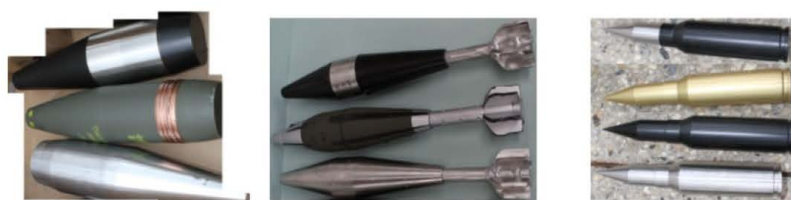
Figure 4. Fabricated surrogates, purchased replicas, and fabricated replicas of (left) 155 mm HE M107, (middle) 81 mm mortars, and (right) 25 mm and 20 mm cartridges (from [13]).
