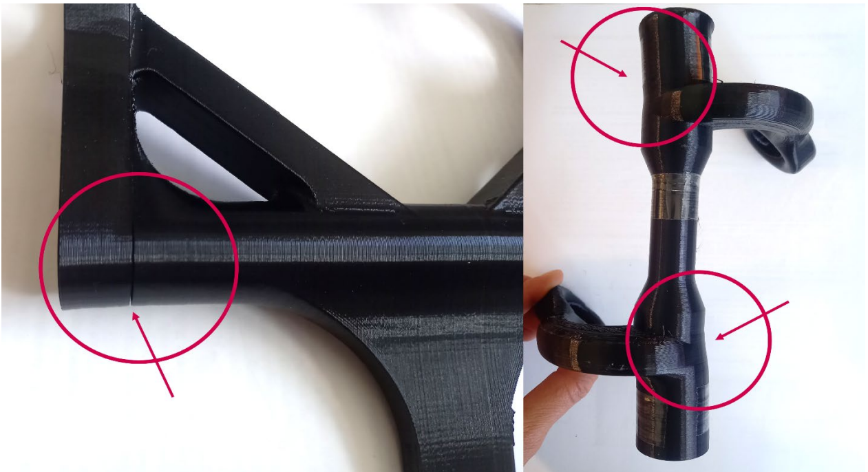
Figure 24: cracked lower handle and bent tube
