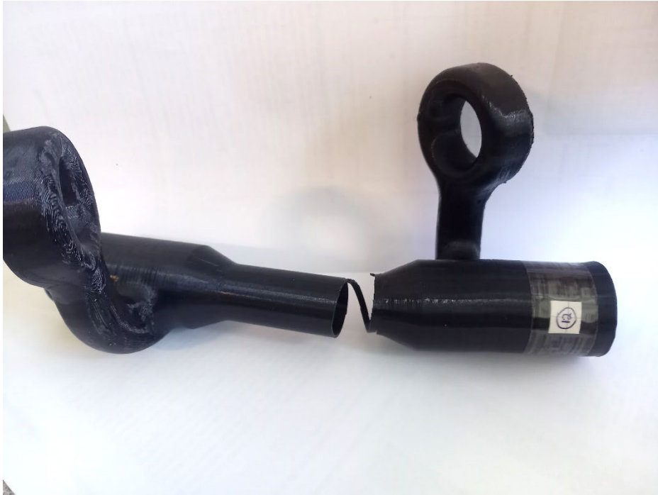
Figure 25: successful test (failed tube, No12)
