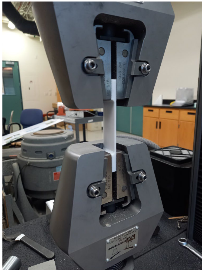
Figure 11: specimen(white) loaded into the tensile testing machine (Instron®)
