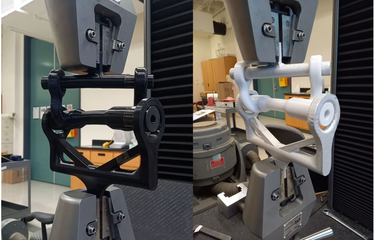
Figure 28: setup for combined loading: PC handles (left) and aluminium handles (right)
