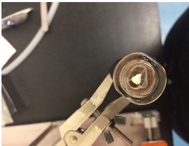
Figure 31. Image of IMX-101 on top of the soil profile during dissolution experiments.
