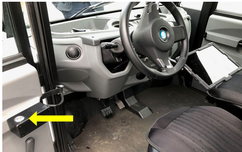
Figure 11. Location of a/m button for switching between manual and autonomous mode.*
