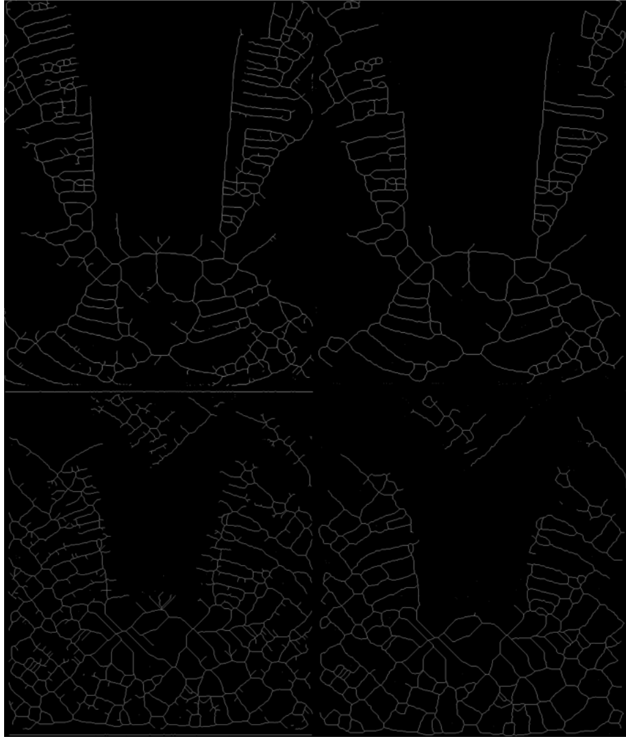
Fig. 4 The images of weak (top) and strong (bottom) impact from the right panels of Fig. 2 were skeletonized with and without pruning the end points, as shown in the right and left panels of this figure, respectively. While pruning the end points is seen to be effective for removing short, artificial line segments that were generated because of noise, there is also the removal of physically relevant features. As such, care should be taken in deciding whether pruning the end points is more helpful than harmful for analyzing the shear band network. The skeletonization of the shear bands results in lines of single-pixel thickness, which may require visualizing under high resolution.
