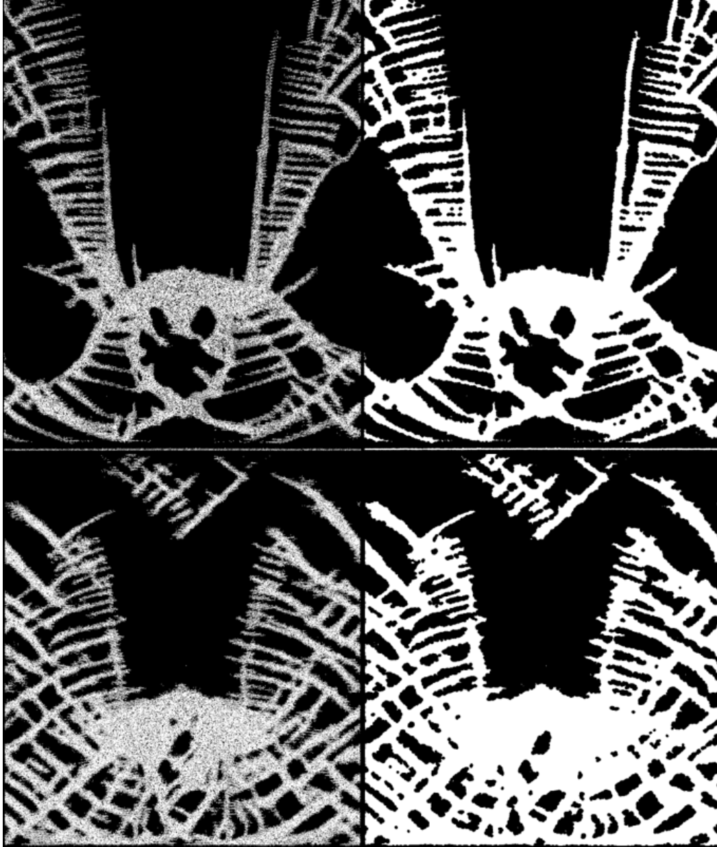
Fig. 2 The two left panels show different shear band structures produced from molecular simulation of RDX pore collapse; the top-left panel used a weak impact velocity while the bottom-left panel used a strong impact velocity. The two right panels show the 8-bit black-and-white images that have been smoothed with the Close– operation using a circular element with a radius of 4 pixels in ImageJ.
