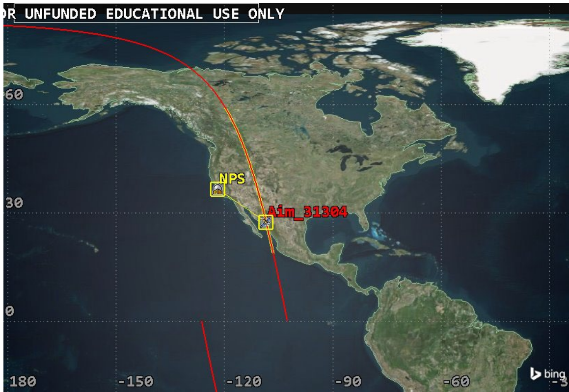
Figure 41. 2-D ground track for AIM-NPS contact
