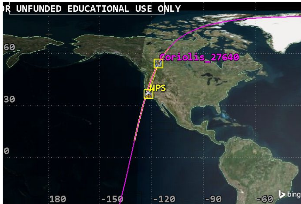
Figure 27. 2-D ground track of Coriolis-NPS contact
