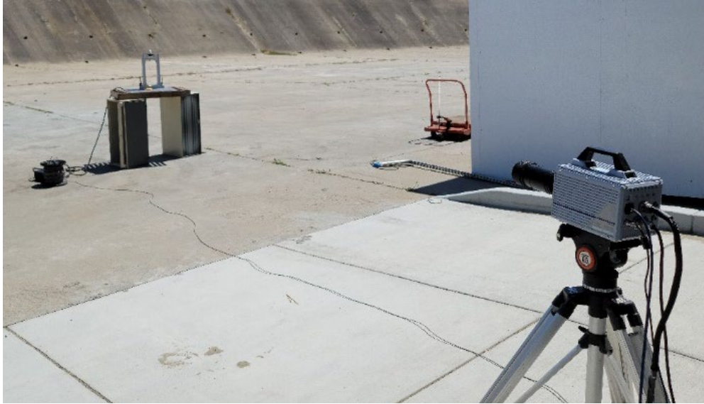
Figure 21. High-speed camera and test stand setup
