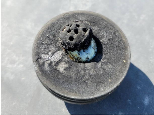
Figure 31. Ignition basket version 2 after live-fire test
