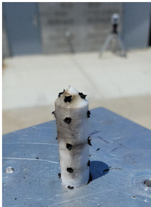
Figure 23. Post-fire 7.62 cm (3 in) basket with clogged holes
