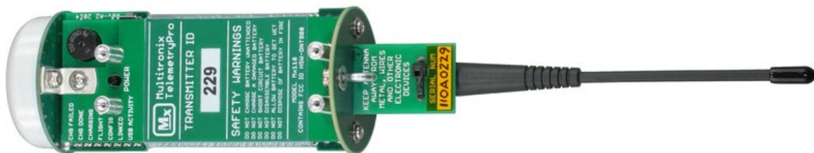
Figure 67. Multitronix Kate-1 TelemetryPro transmitter. Source: [25].
