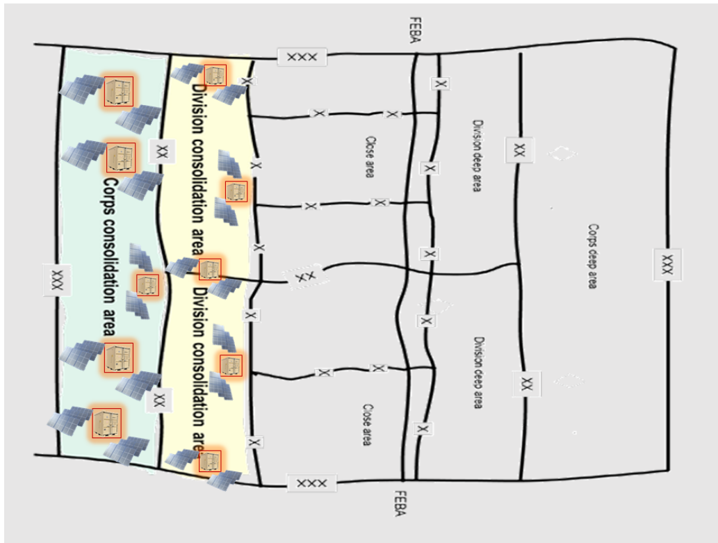
Figure 2.5. Mobile Microgrid CONOPS for Large Scale Combat Operations: This CONOPS for LSCO shows a simple operational graphic, taken from Army FM 3.0, for LSCO with the potential areas of the battlefield where mobile microgrids could best be used. The idea is to reduce fuel consumption in the rear-echelon formations to allow logistics assets to focus toward the forward edge of the battle area. Adapted from [42].
