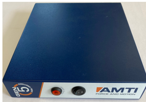
Figure 2.6. AMTI Gen 5 Amplifier used for the dynamic validation and experimental measurements.
