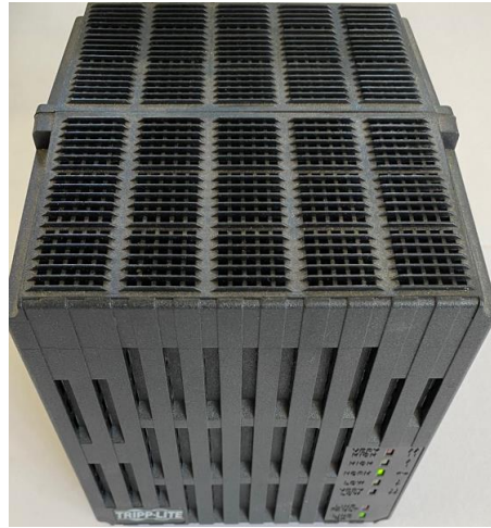
(b) AC power supply unit
