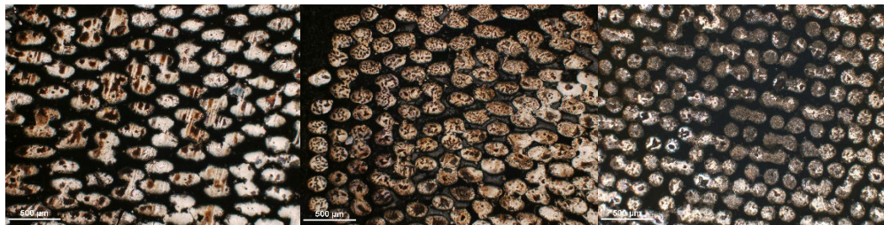
Figure 54. Variation in pillar geometry with CNT concentration (pure SS [a], 1 vol. % CNT [b] and 2 vol. % CNT [c])
