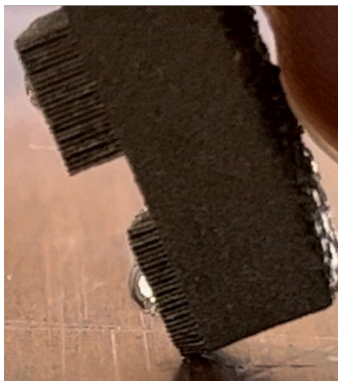
Figure 47. Water roll-off angle test for 1 vol. % CNT SS sample
