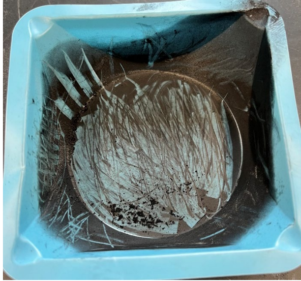
Figure 17. Residual carbon in 5% CNT milling process
