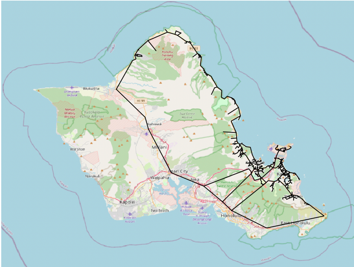
Figure 3.7. Skeletonized Road Network. A simpler road network is necessary for our model to run efficiently. This was done by removing any unnecessary vertices in the network to simplify the shape of the roads and remove extraneous variables from our model.
