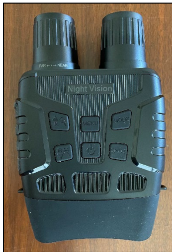
Figure 28. Night vision device with video and photo recording capability
