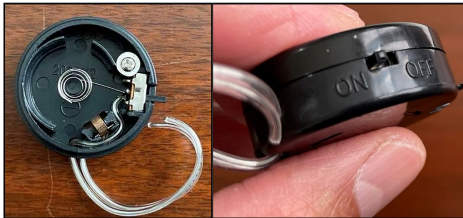
Figure 8. Battery case with ON/OFF switch
