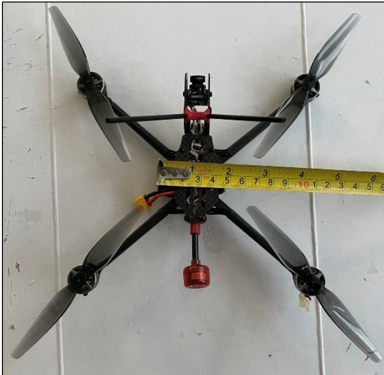
Figure 1. 50 mm workspace on a sub-250 gram quadcopter
