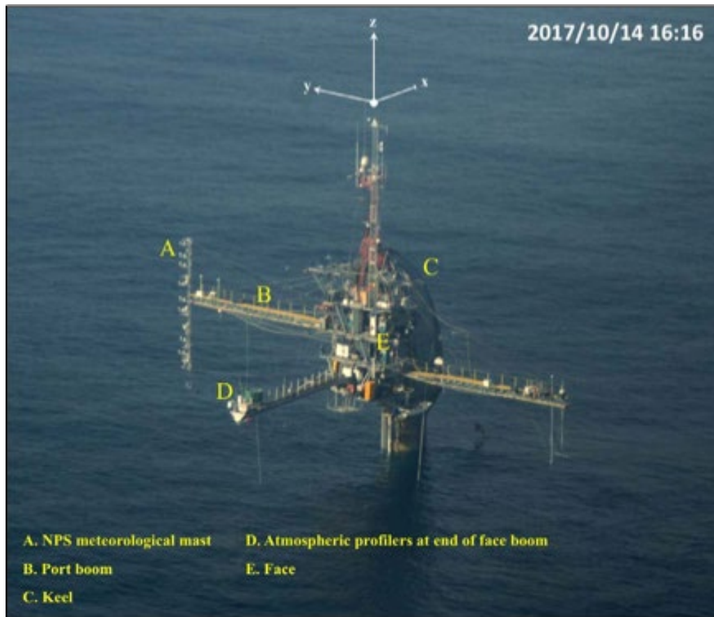
Figure 5. Image of R/P FLIP during the 2017 CASPER-West experiment with key features identified. Source: Ortiz-Suslow et al. (2019).
