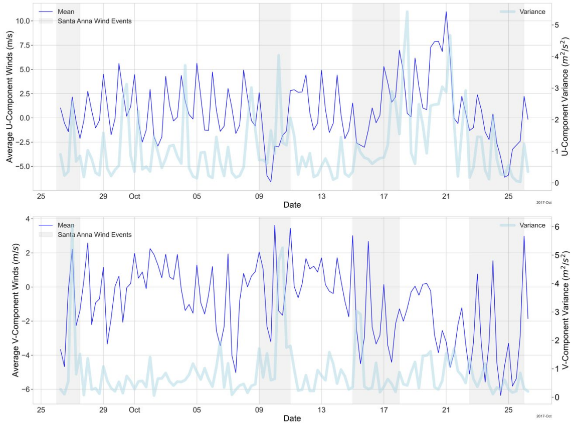
Figure 24. Time series plot of the simple mean TLMM average and variance. Values are averaged over all platforms; i.e., calculations do not differentiate observation locations.
