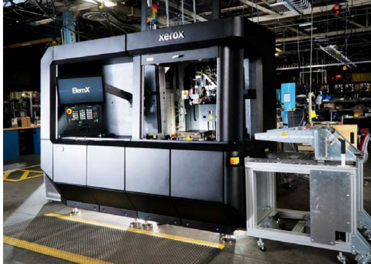
Figure 2. Xerox ElemX Liquid Metal Printer with Build Plate Transfer Crane. Source: [6]
