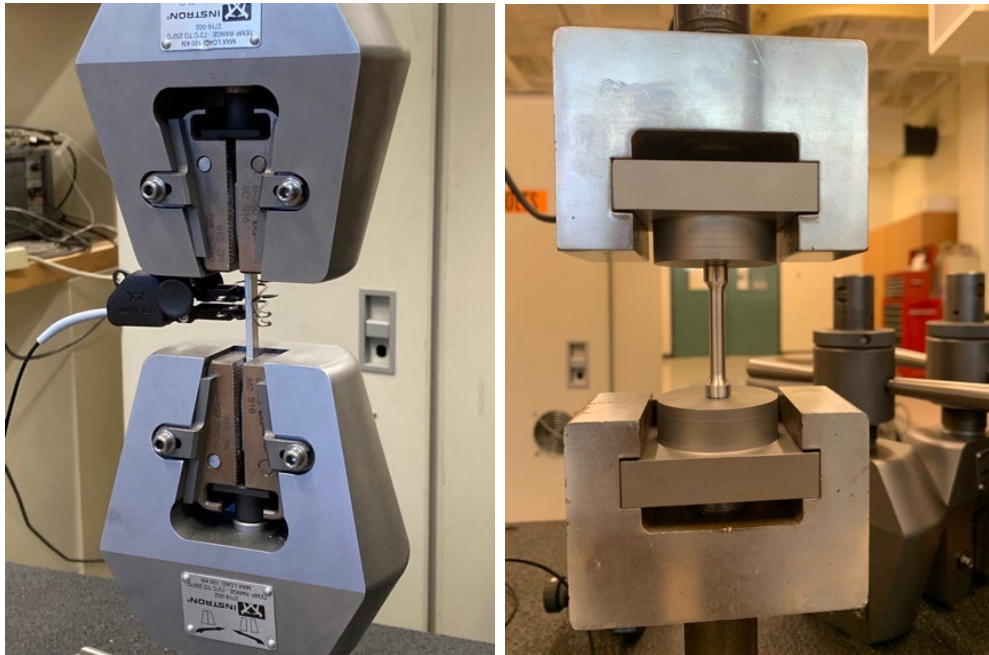
Left: As-printed tensile specimen. Right: Printed block then machined circular cross-section tensile specimen.
