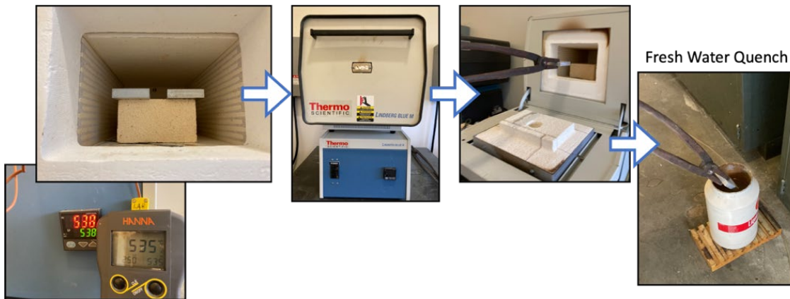
Figure 19. Solution Treatment Process
