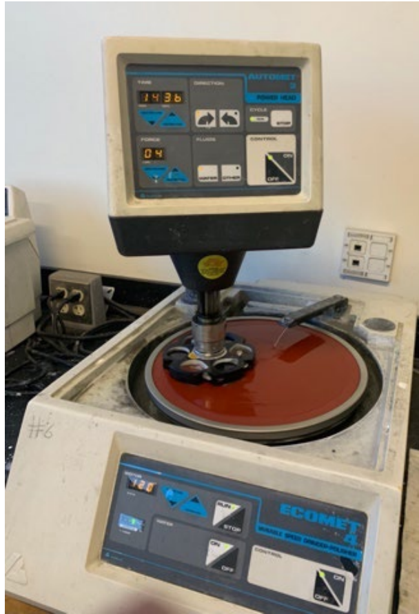
Figure 23. Ecomet4 Variable Speed Variable Speed Grinder/Polisher Used to Prepare the Samples for Microscopy and Microhardness Testing
