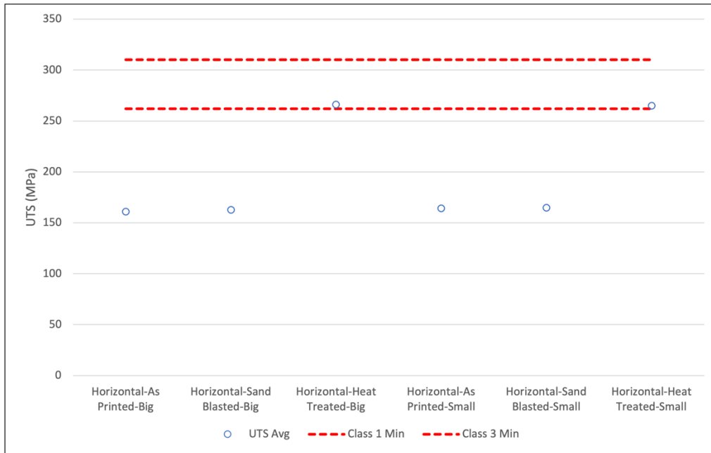
Figure 41. Ultimate Tensile Strength: Heat Treated and Sand Blasted Printed Tensile Specimens
