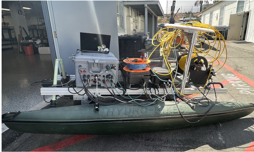
Figure 6.6. The following image is a visual depiction of the physical CASSMIR USV platform used for our thesis use case.
