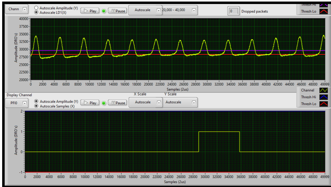
Figure 16. Live Data Tab Showing Live Capacitive Probe and Tachometer Signals.
