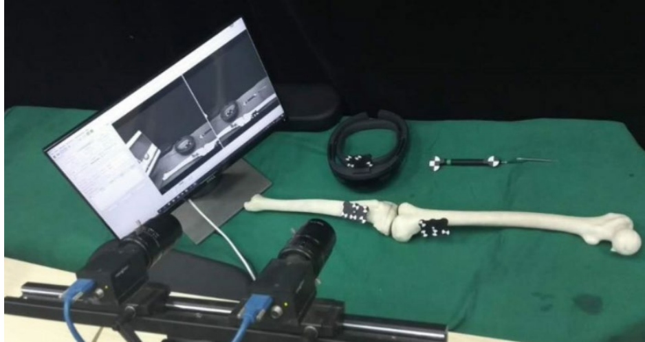
Figure 7. The Experimental Scene of Wang et al. Note the positional markers on the objects as well as the binocular camera used to calibrate their respective locations. Source: Wang et al. (2019).
