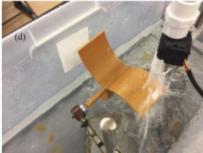
Figure 1.14. Number of Blades and Curvature Drag Turbine Experimental Set-up. Source: [16].
