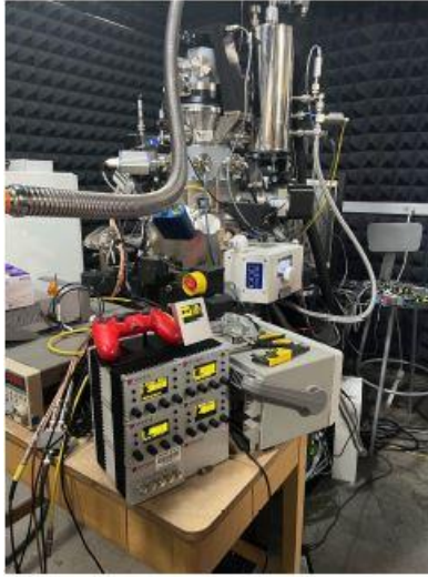
Figure 8. Zeiss Orion Helium Ion Microscope, where Helium ion beam with different dosage was utilized to pattern YBCO film in a nano-meter scale.
