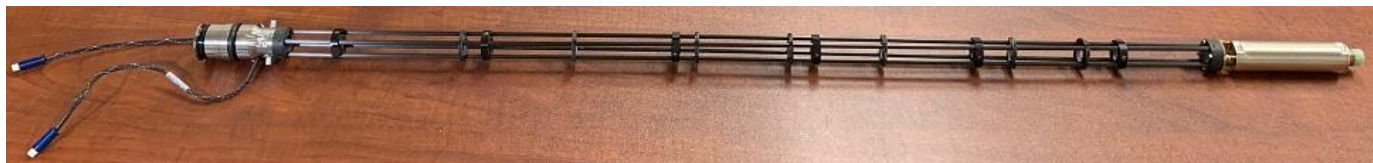
Figure 2. Cryogenic OMFP probe for high T_c SQUID detection.
