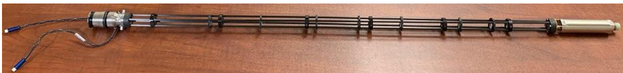
Figure 6. OMFP specifically designed for High T_c SQUID application.
