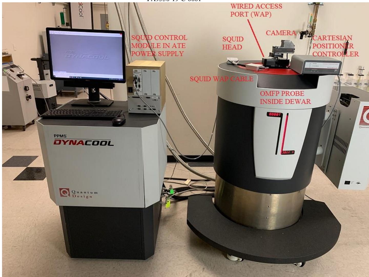
Figure 1. High T_c SQUID System Set-up in QD's Dynacool System, where a cryogenic probe (OMFP) is inside the sample space in the dewar.
