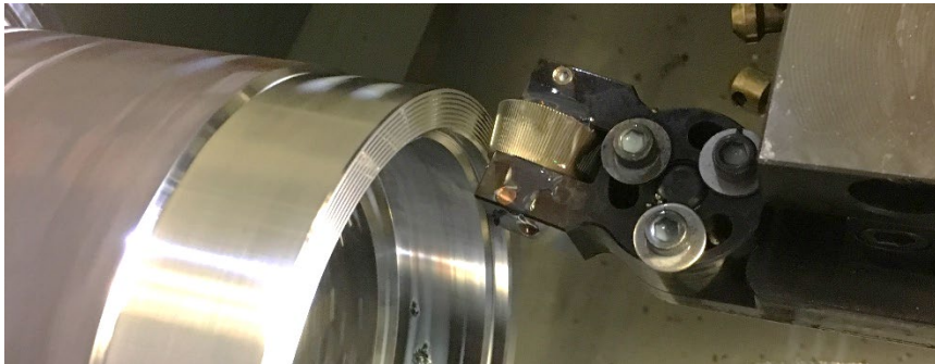
Figure 4 A prototype 20-TPI knurling wheel imprinting on the face of a test item
