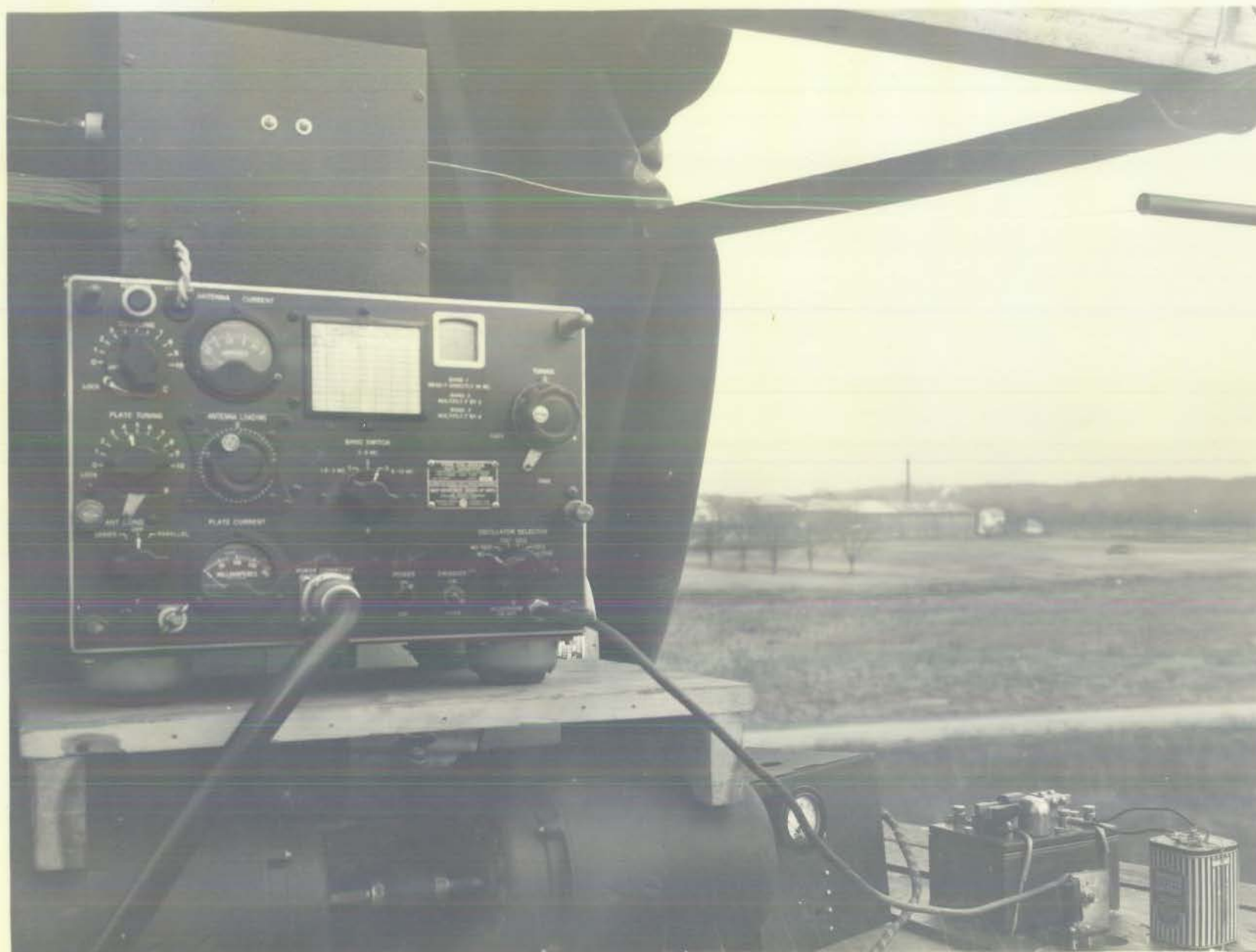
TCS-5 TRANSMITTER (SHOWING ELECTRIC POWER SUPPLY AND MODULATOR)
