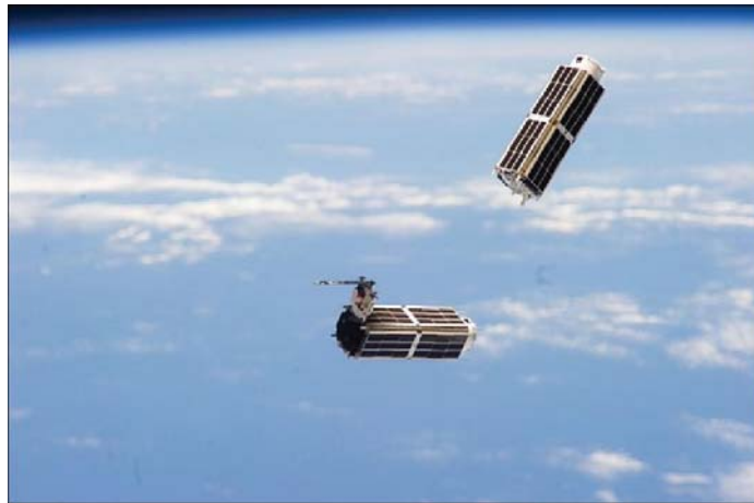
Figure 8. Deployment of First Two Flock 1 Cubesats. Source: [26].
