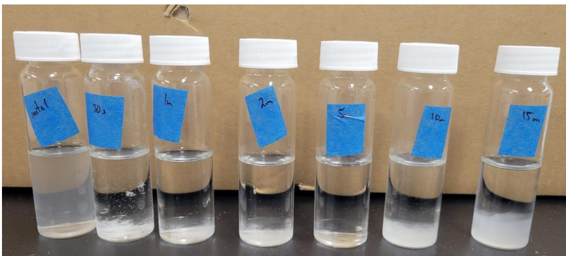
Figure 8. Floc formation from oily wastewater with surfactant as seen in samples taken over 15 minute.
