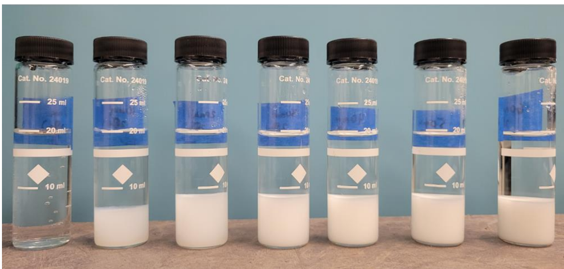
Figure 4. Images showing precipitate formation immediately after the conclusion of an experiment (top) and after allowing for floc development (bottom).
