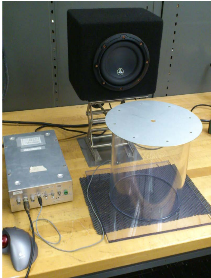
Figure 20. Experimental setup for determining resonance frequency of an approximately neckless cylindrical Helmholtz resonator
