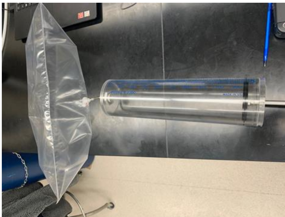
Figure 8: Transferring critically measured contents from 2-liter gas tight syringe through a 1.5-inch tube, into a 10-liter Tedlar® bag.
