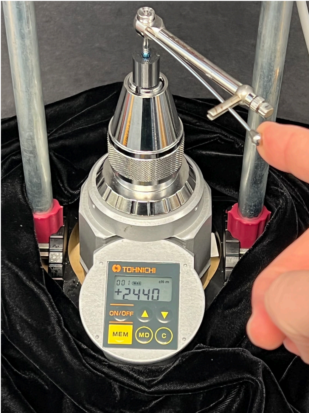
Figure 4. Hand Torque Wrench measuring the final torque value of the implant in the polymer to compare to the present torque value on the implant motor
