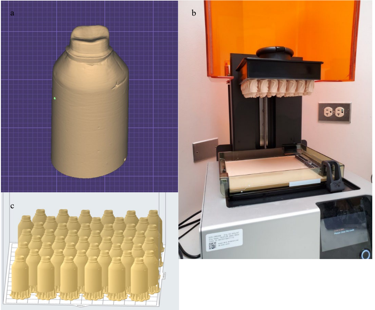
Figure 2. a-c: Digital workflow for fabrication SLA (3-D printed) dies (Image c credit to MAJ Migdalia Torres).
