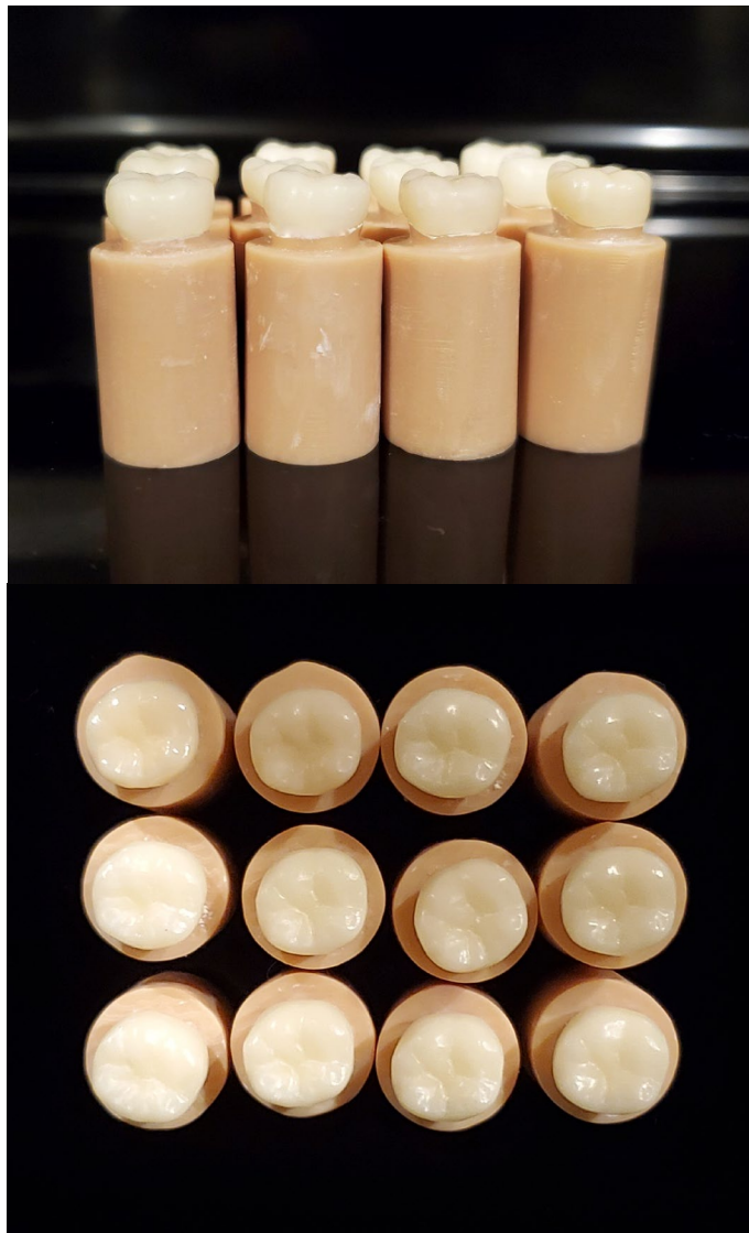
Figure 3. Provisional crowns cemented to SLA fabricated dies (Photos credit to MAJ Migdalia Torres).
