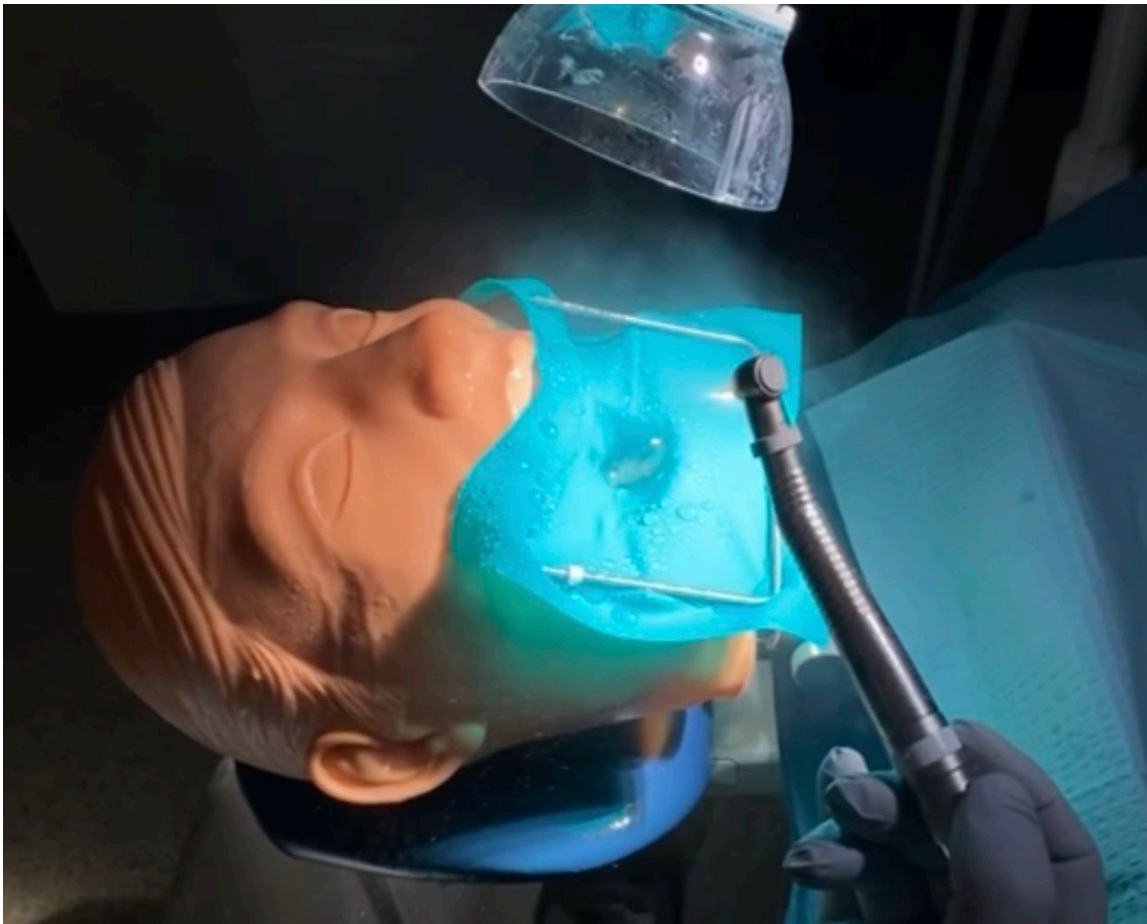
Figure 6. High Speed Handpiece Aerosol Production. Visual representation of aerosol/spatter production by the NSK-NL-85M high speed handpiece (444,000 rpm, 88ml/min). No mitigation devices in use. The PAX 2000X unit pictured is not operating (power setting set to off) at the time of the photograph. The handpiece was held away from the working field (tooth #19) for visual, photographic demonstration.
