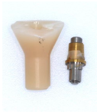
Figure 5. Post testing. (a) Conventional Ti base, (b) Screw channel correcting Ti base
