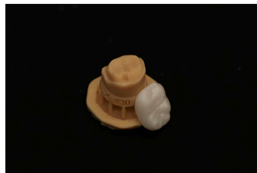
Figure 6: Die model from digital die trimming and milled Zenostar Translucent Zirconia crown from 3Shape Automate CAD file.
