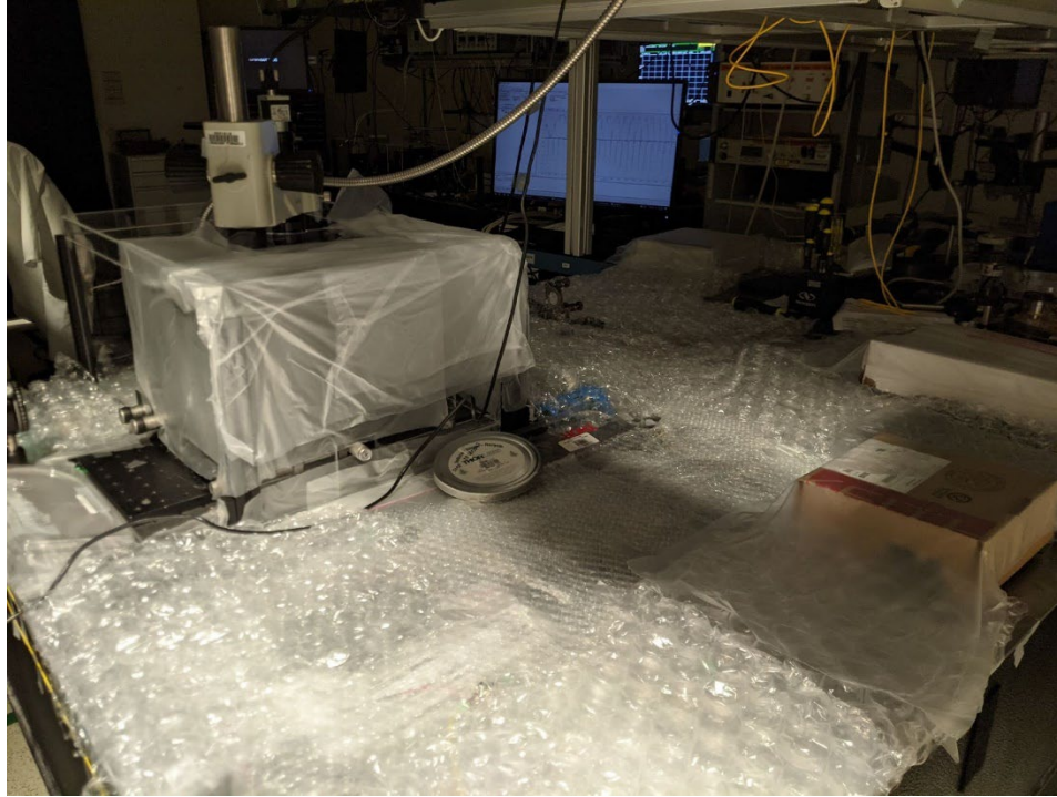
Figure 8: External Measurement Setup with Fibers Require Extensive Packing Material to Ensure Temperature/Air/Humidity Isolation for Phase Measurement in Ring Resonators
