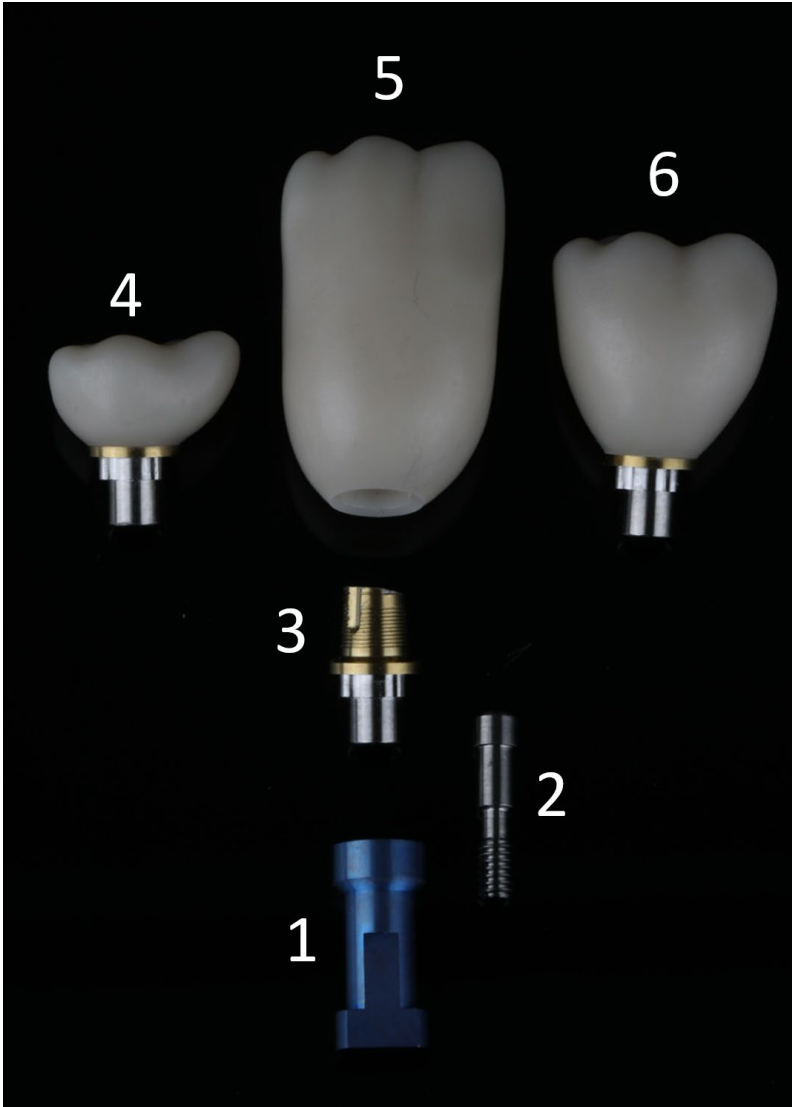
Figure 3. Test Group Components. Assembly of hybrid abutment crown test groups. (1) Laboratory implant analog. (2) Titanium screw (3) Tibase (MIST L-Link; Imagine USA, Chantilly, VA) cut to 4mm in height. (4) Completed 6mm zirconia crown cemented to the Tibase. (5) Milled 19.25mm zirconia crown prior to cementation to the Tibase. (6) Completed 12mm zirconia crown cemented to the Tibase.
