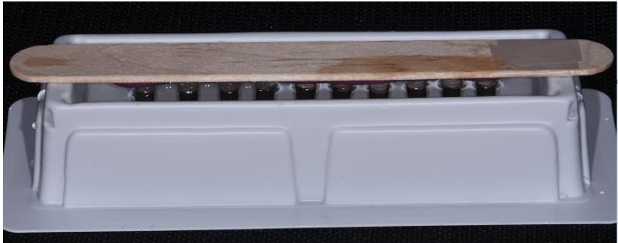
Fig. 5. Implants were immersed in the inoculum suspension in a way that only the coronal 6 mm of the implant surfaces were exposed.
