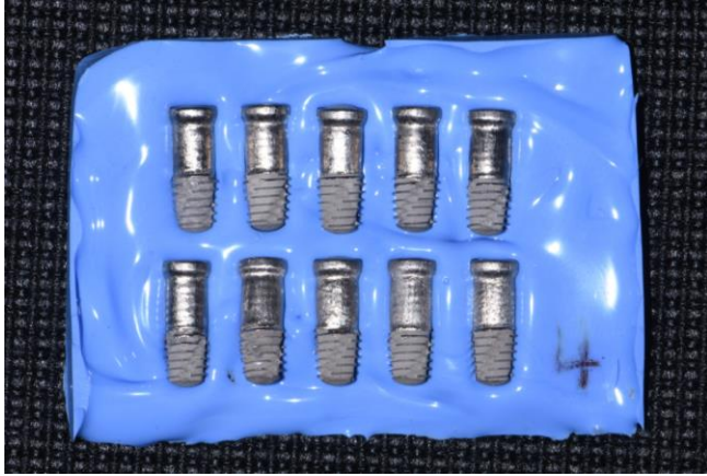
Fig. 2. Each group was fixed into PVS impression material to stabilize the implants
