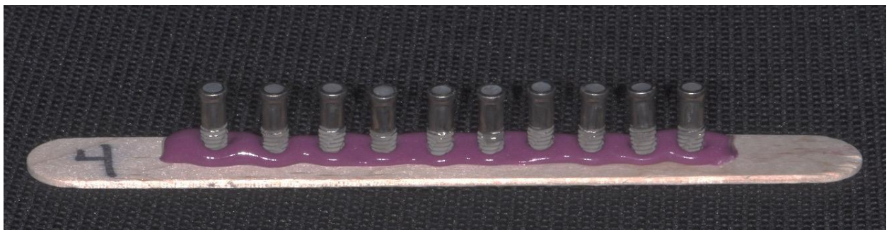
Fig. 4. Implants were secured on a tongue depressor with PVS impression material to facilitate immersion in inoculum suspension (see Fig. 5).
