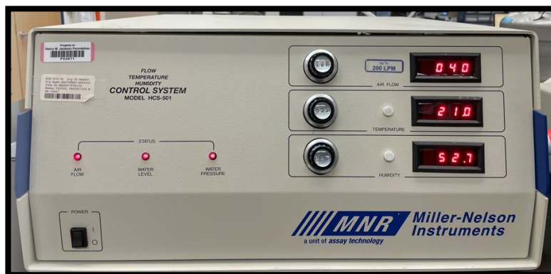
Figure 7: Miller-Nelson HCS-501 front panel with airflow, temperature, and humidity display.
