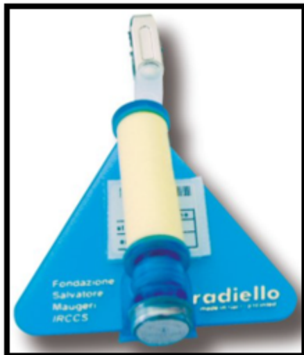
Figure 2: A Radial Diffusive Sampler: Radiello® C-RAD145 sampler with the yellow diffusive body packed with Carbograph 4 adsorbent (18; 38)
