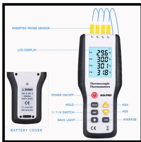
Figure 15: Risepro 4-Channel Digital Thermocouple Thermometer with four sensors (46).
