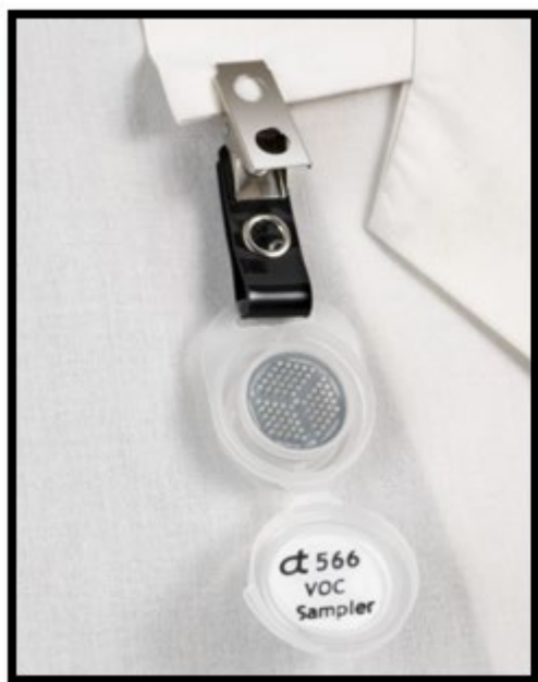
Figure 1: An axial diffusive sampler: The Assay Technology 566 OVM sampler with an inert charcoal wafer and 76-hole sampling grid (17; 38).
