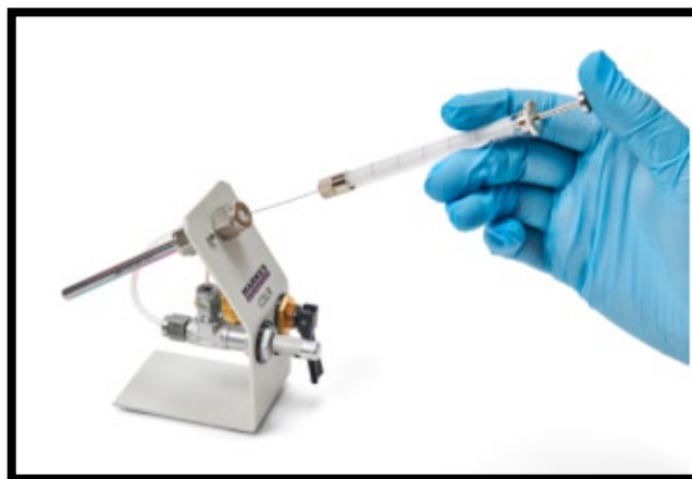
Figure 31: Loading one \mu\text{L} of liquid benzene into CSLR (33).
