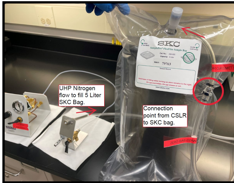
Figure 43: CSLR connection to fill the 5 Liter SKC bag with UHP Nitrogen.
