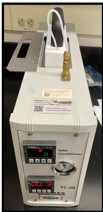
Figure 25: TC-20 with tube manifold block loaded with TD tubes for conditioning.
