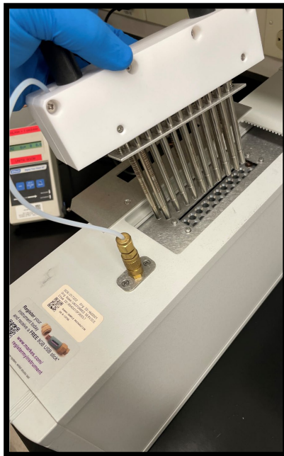
Figure 25: TC-20 with tube manifold block loaded with TD tubes for conditioning.
