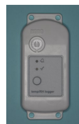
Fig. 3. Data logger used to record hourly temperatures
