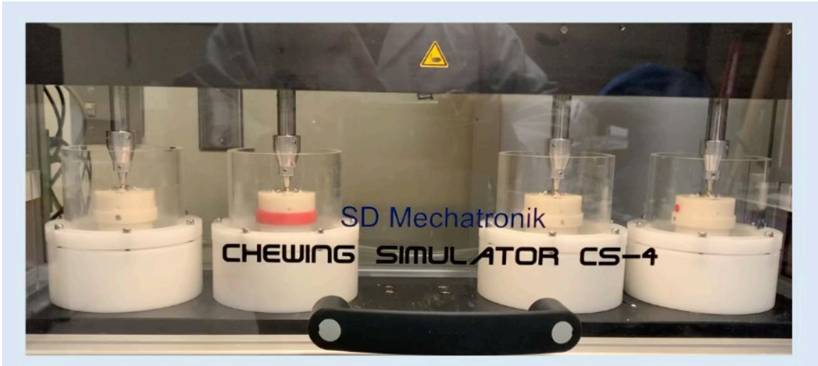
Figure 8. Four Samples Mounted in the Chewing Simulator.
