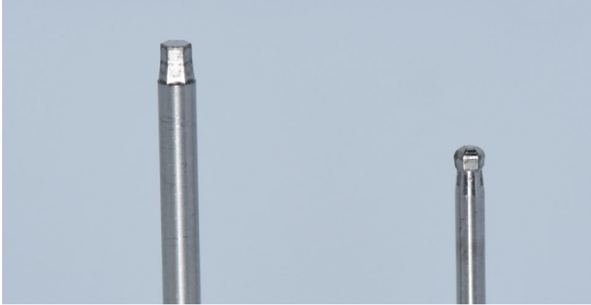
Figure 4. Hexagon Driver and Hexalobulated Driver.
