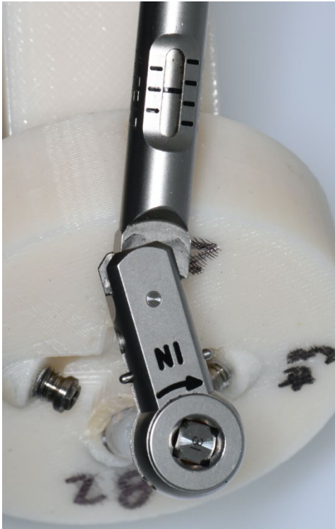
Figure 6. Torque Wrench Action at 20 Ncm.
