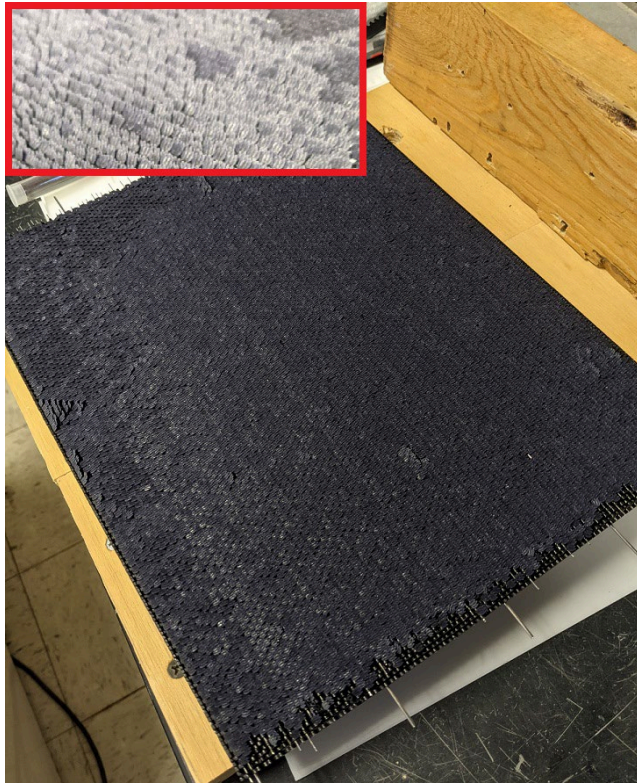
Figure 9: MAKO model for water tunnel testing before mounted into a flat plate.. The plate contains over 9,000 3D printed scales assembled by hand each 3.7 mm in size. Enlarged image (red) shows a closer up view of the scales with some of them bristled to their maximum angle. This model used black plastic printing material as the black matte finish is best to use with DPIV and minimize laser reflection.
