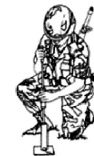
Applying drop hammer blows with the remolding equipment.
