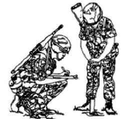
Measuring cone index in the remolding cylinder before and after hammer blows.
