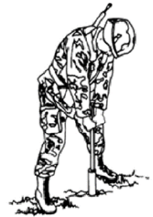
Using the sampler to obtain a soil sample for a remolding test.
