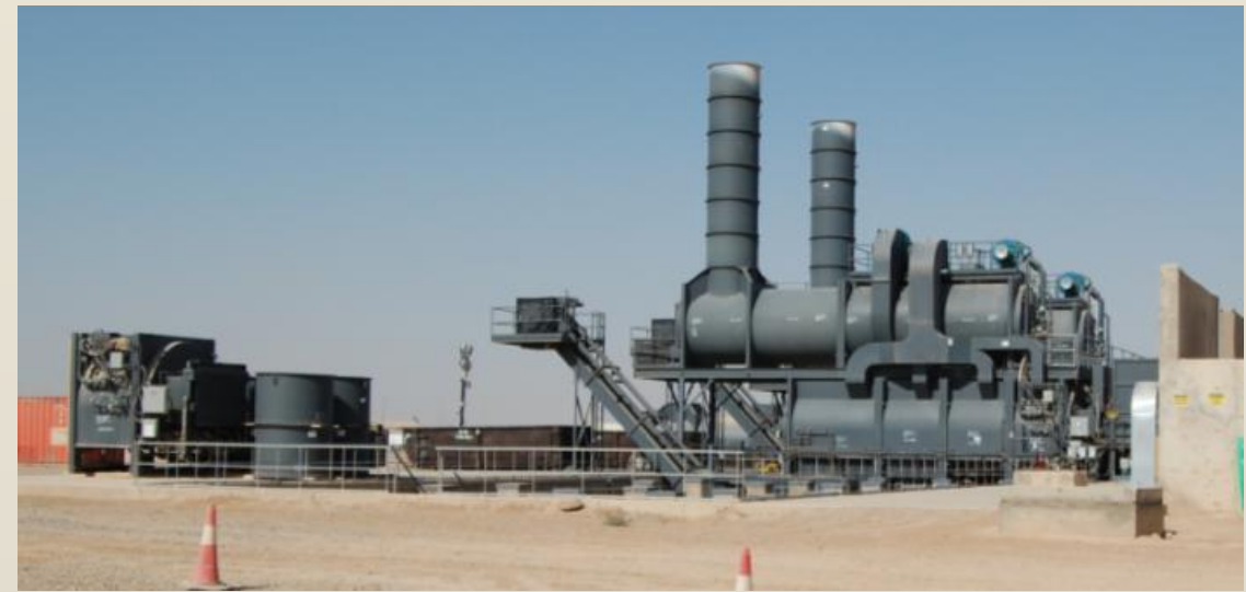
Two 64-ton Solid Waste Incinerators Typical burn temperature 1500-1800° F
