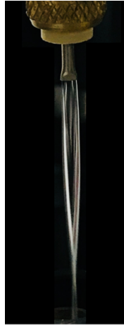
Fig. 9 Photo of a 120 \mu\text{m} thick water film formed by a water jet with a flat nozzle. The laser beam is focused into the center of the film where is flat and stable.
