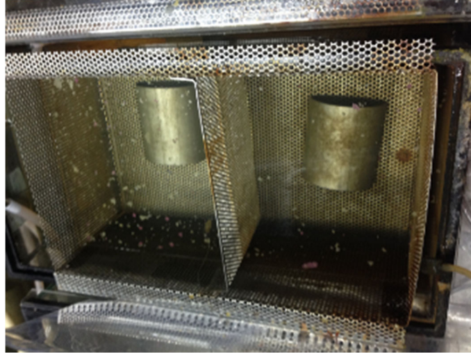
Figure 5. Mesh cage with partition for housing Cyprinodon variegatus in experimental mesocosms.
